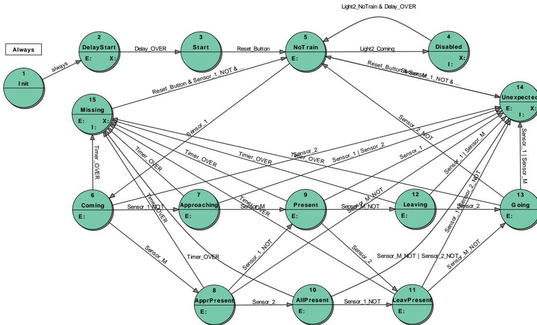
The state transition diagram displays only the states and transition conditions. The complete specification requires the entry, exit and input actions which are only indicated in the diagram by letters E, X, I. The full specification is included in state transition tables. (If you explore the design by means of StateWORKS Studio, you will need to double-click on any state to see the full details of its actions and transitions.)
