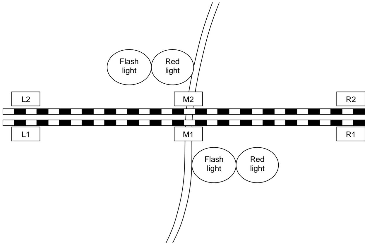
The railway consists of two tracks. Each is monitored by three sensors L(left), M(middle) and R(right).
