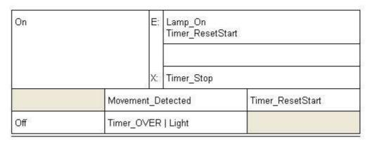
Figure 4 Security lamp: State transition table of the state On
