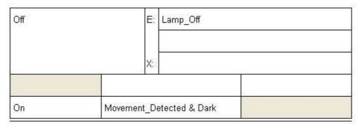
Figure 3 Security lamp: State transition table of the state Off
