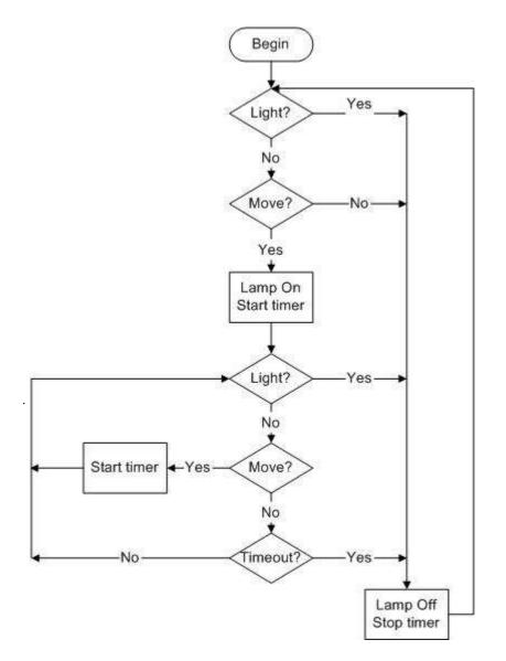
Figure 5 Flowchart of the Security lamp control
