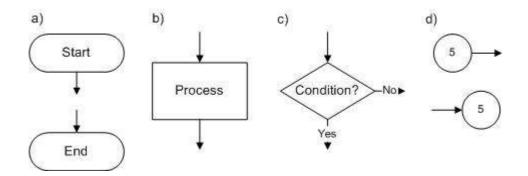
Figure 1 Flow chart symbols: a). Start and End; b). Activity; c) Decision; d). Place marker (to show links between two places of a flowchart)
