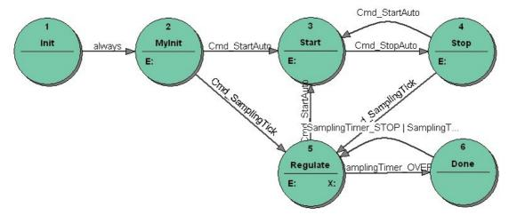
Figure 1: PID Test: State transition diagram
